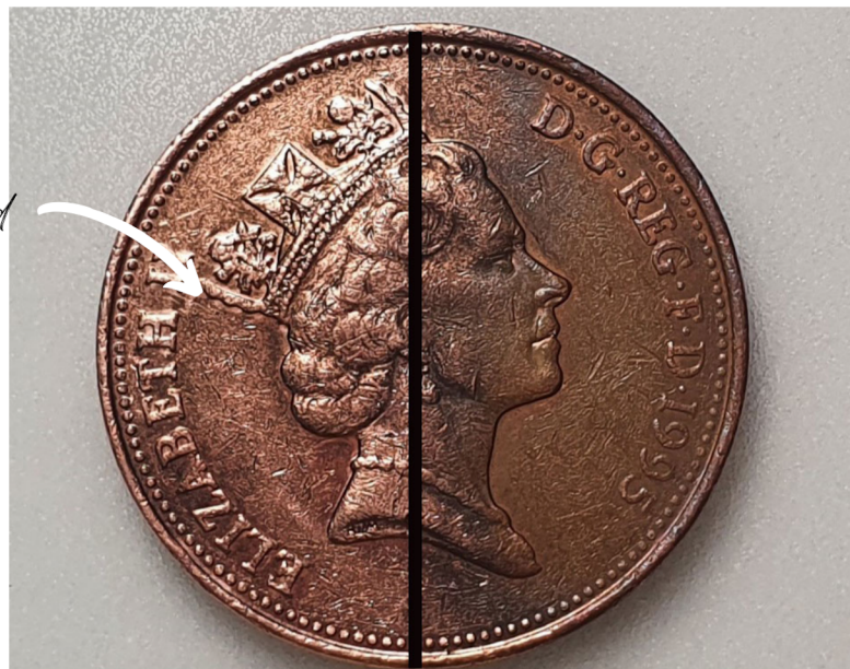
50:50 Water vapor plasma treated coin
